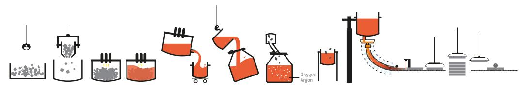
Using an electric arc furnace with a **melting capacity of up to 160 tonnes**, the **raw material** (recycled stainless and ferro alloys) is transformed into **molten metal**.
