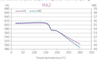
$<sup>^{(5)} \, \</sup>text{Austenitisation for 10 minutes at } 1025^{\circ}\text{C} \, - \, \text{Forced air cooling to } 20^{\circ}\text{C} \, - \, \text{Tempering for 1 hour at } 180^{\circ}\text{C}.$
